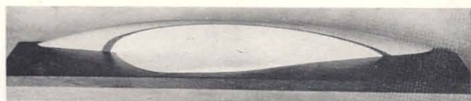
Fig. 16. Painted model of the twelve meter boat Matena as seen from below
