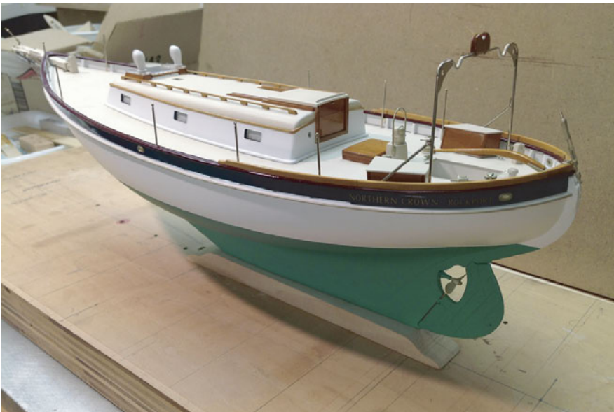
Northern Crown Stern view of model with boom gallows, bulwarks and railcap
