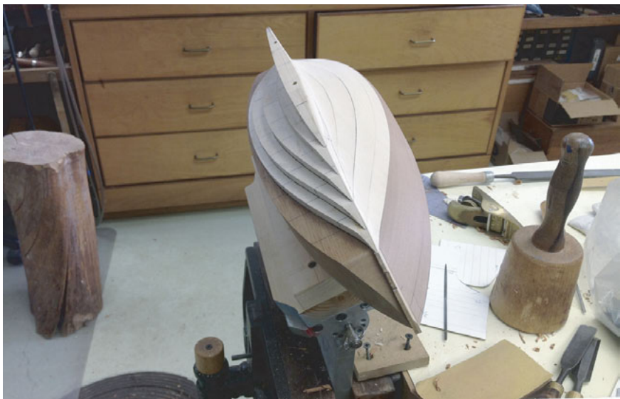
Port side carved away with model mounted on our custom designed carving jig
