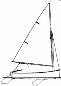
La Petite (11'5" x 4'5") is a lapstrake frostbite dinghy whose spars can fit within her hull. Winter racing gave rise to similar dinghies from various designers. Catalog No. 38.172
