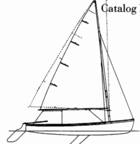
So and So (15'0" x 4'7") can be rowed as well as sailed, with the rower astride the seat that runs fore and aft atop the centerboard trunk. Catalog No. 38.174
