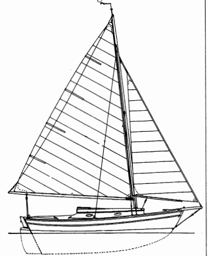
H-23 (22'9" x 8'0") is a small, shallow-draft keel cruising sloop for two, drawn originally for The Rudder as a "how-to-build" article. Catalog No. 38.95
